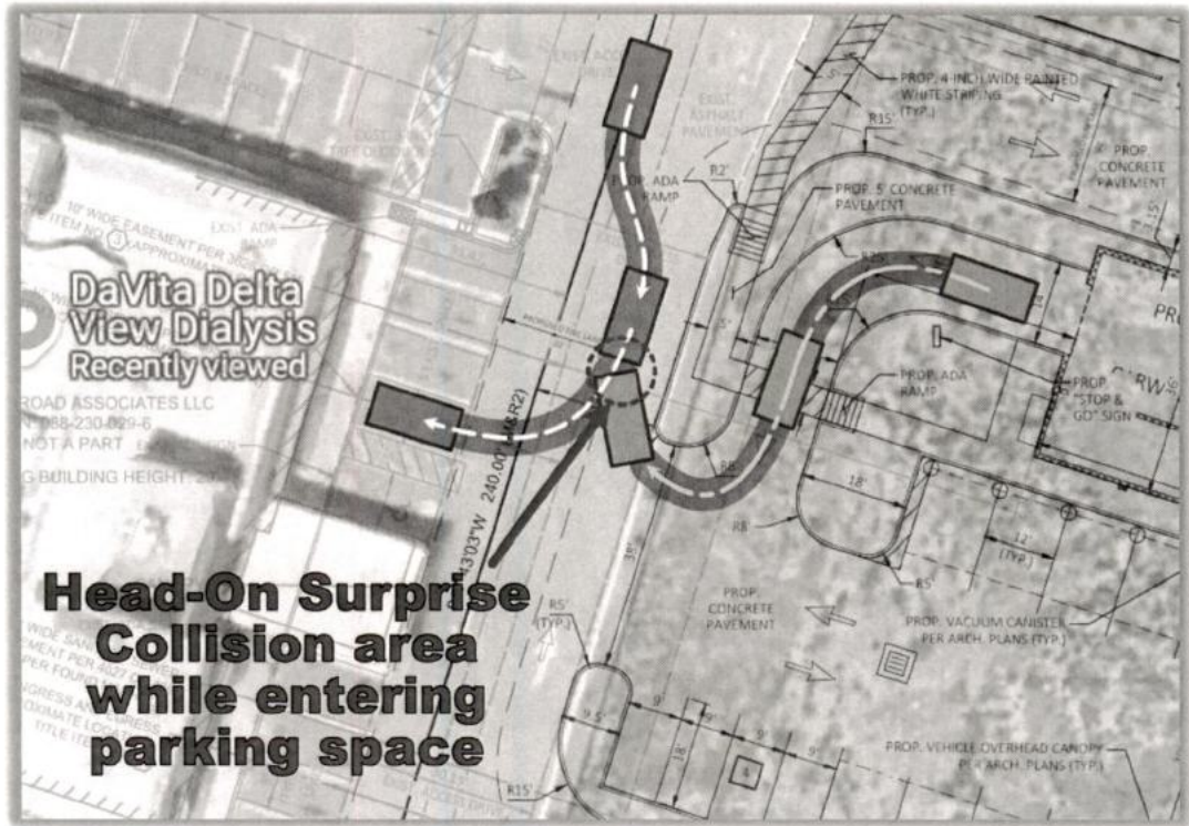
Figure 3. Parking Maneuver INBOUND at Intersection #2 on Figure 1. Significant hazard with turns from new connection due to blind spots and unexpected motions of vehicles, typical of many locations on Delta View Center site.
