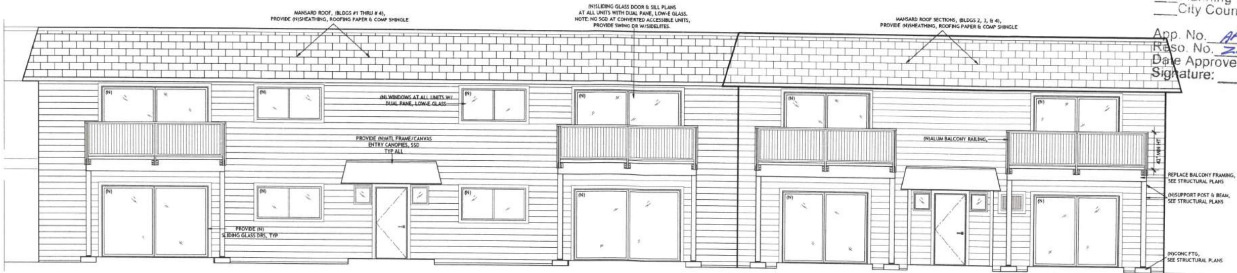
PROPOSED EXTERIOR ELEVATION: (N) LAP SIDING OVER (E) T1-11 (BLDGS. #4 THROUGH #15; BLDG. #3 SIM)
