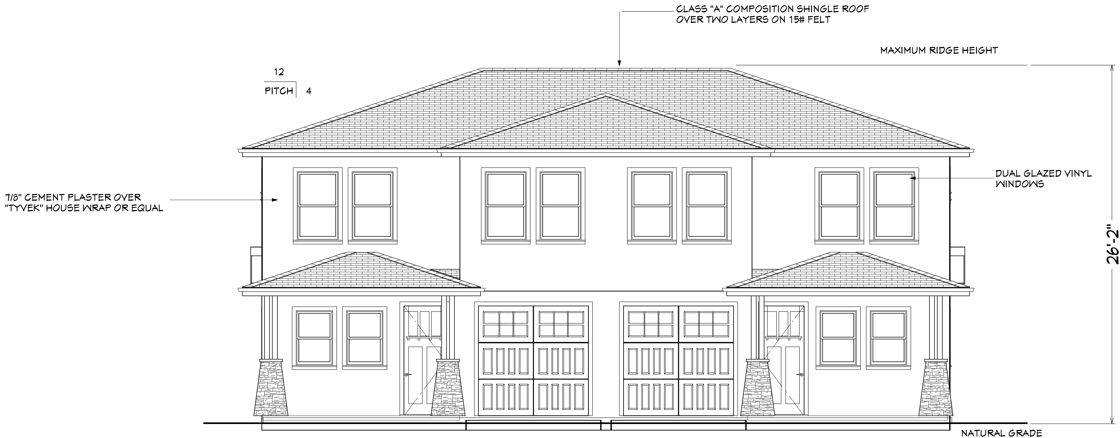
Front Elevation Unit 1-2 1/4" = 1'-0"
