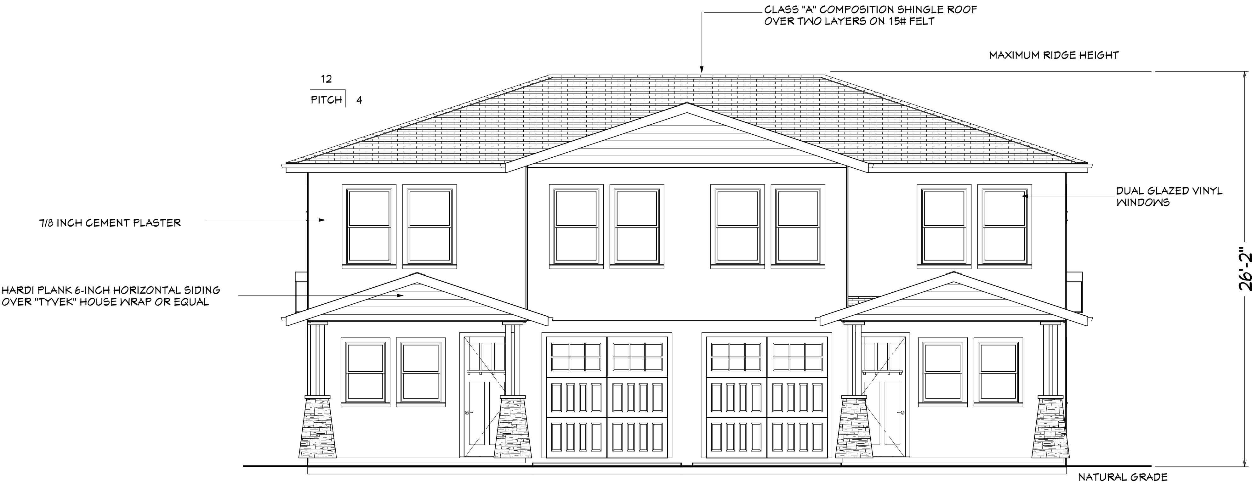
Front Elevation Unit 1-2 1/4" = 1'-0"
