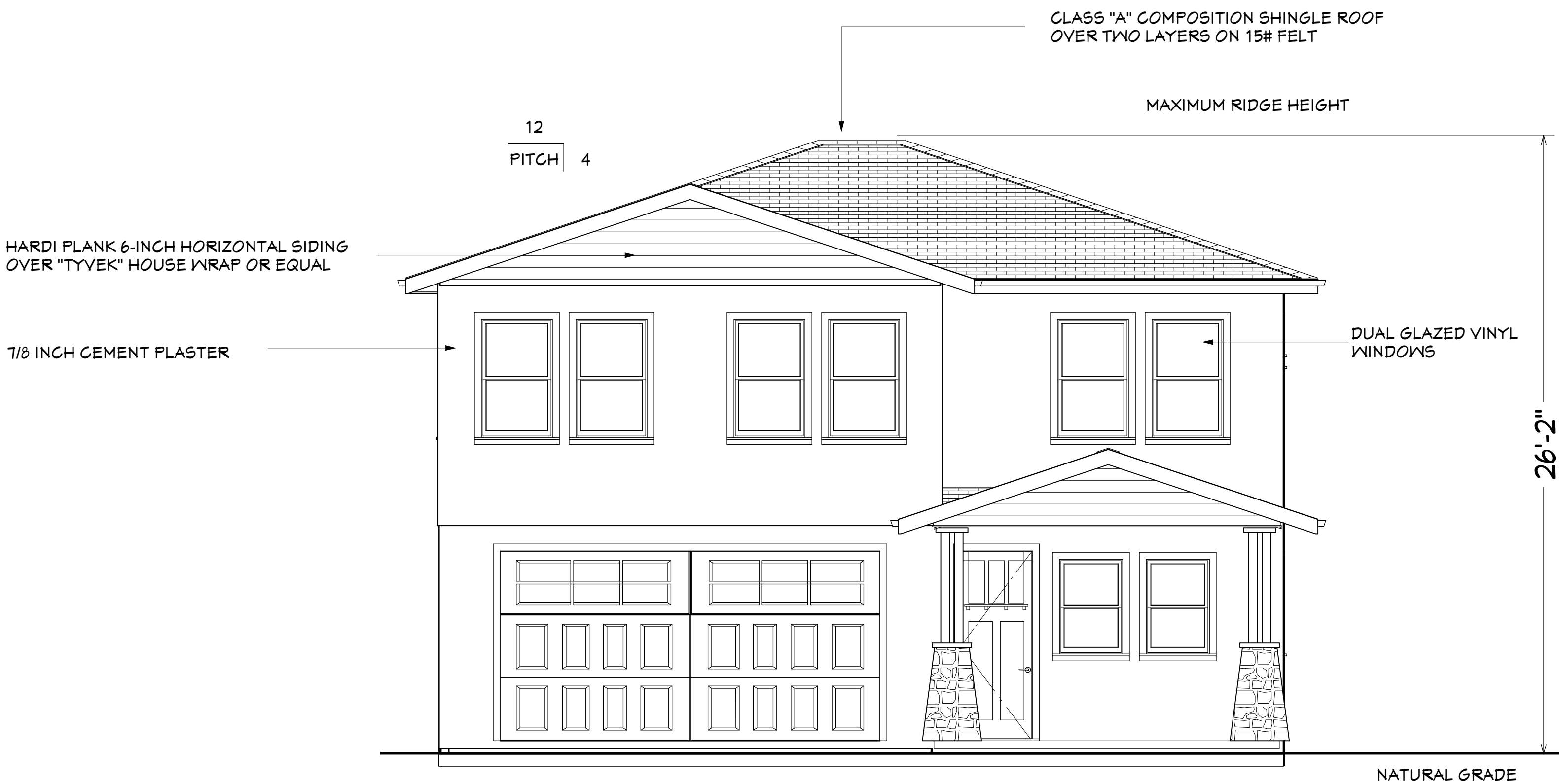
Front Elevation Unit 3 1/4" = 1'-0"
