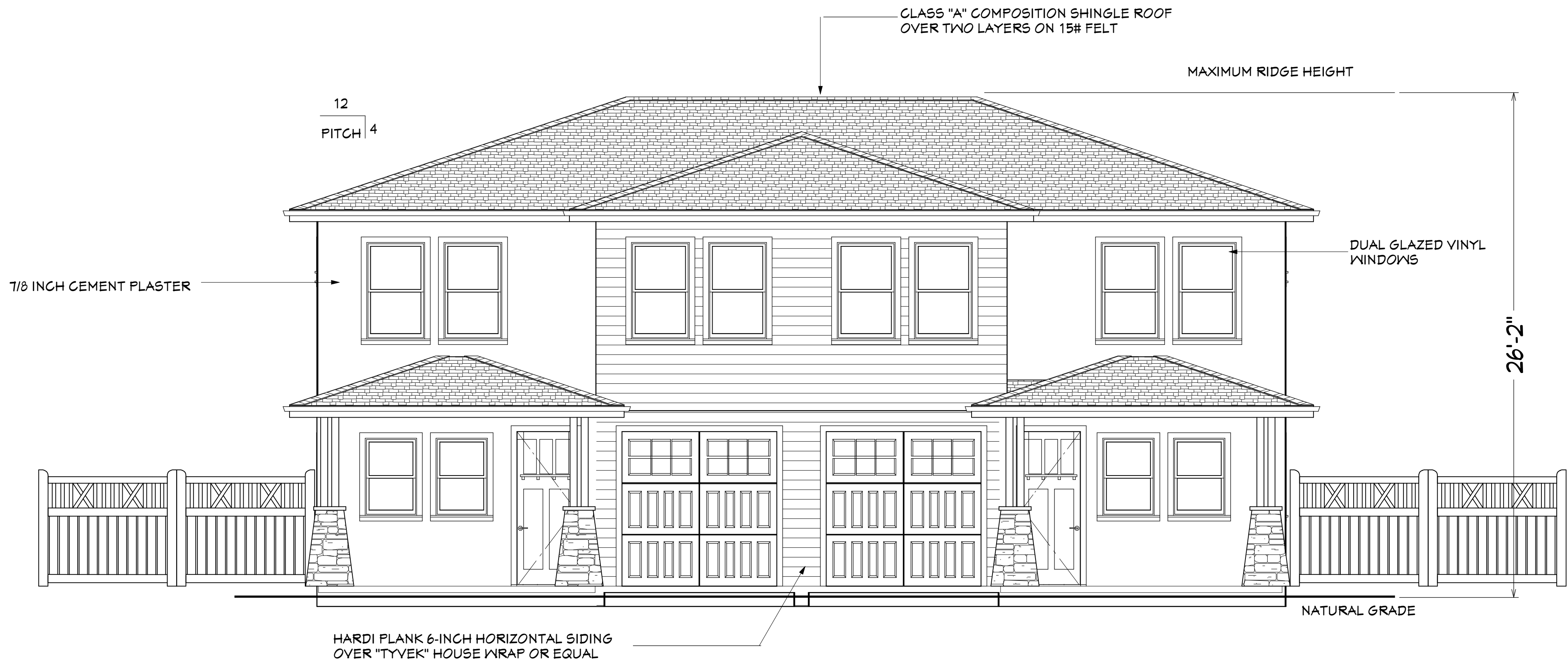
Front Elevation Unit 1-2 1/4" = 1'-0"
