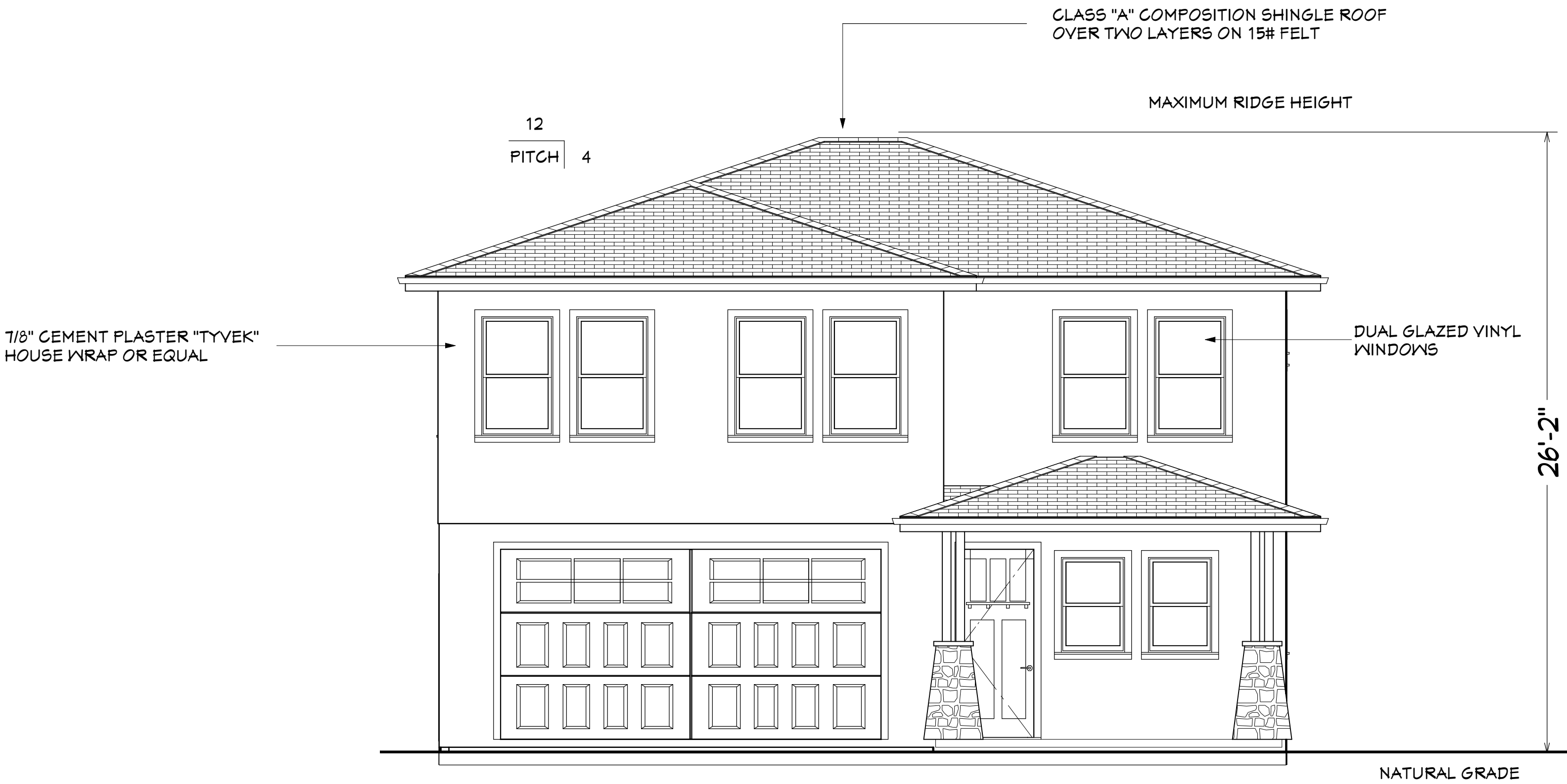
Front Elevation Unit 3 1/4" = 1'-0"
