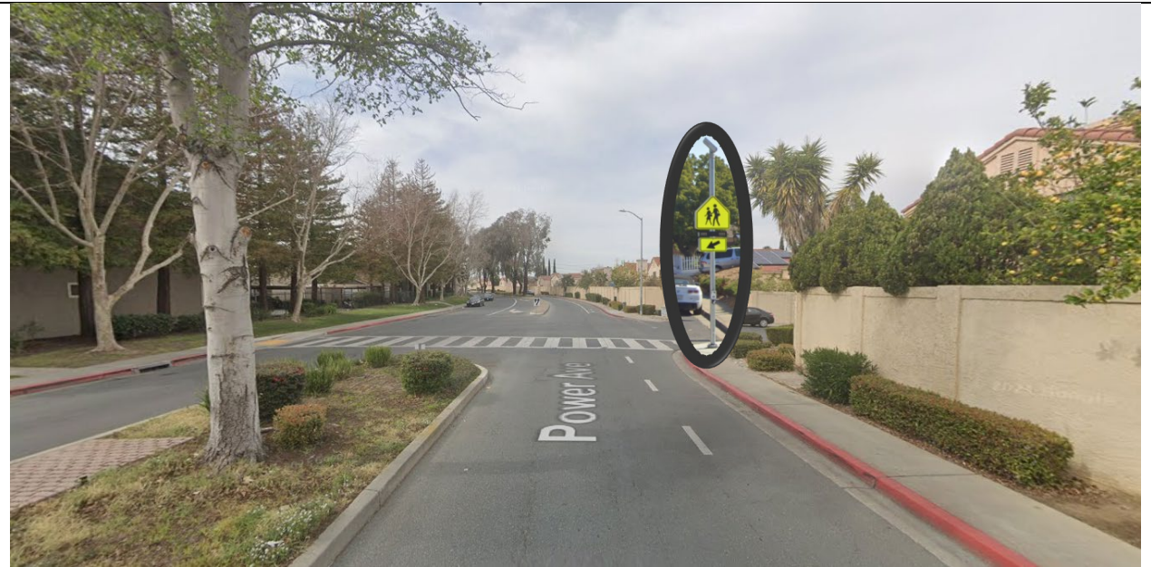
Example of Proposed RRFB to be Installed
