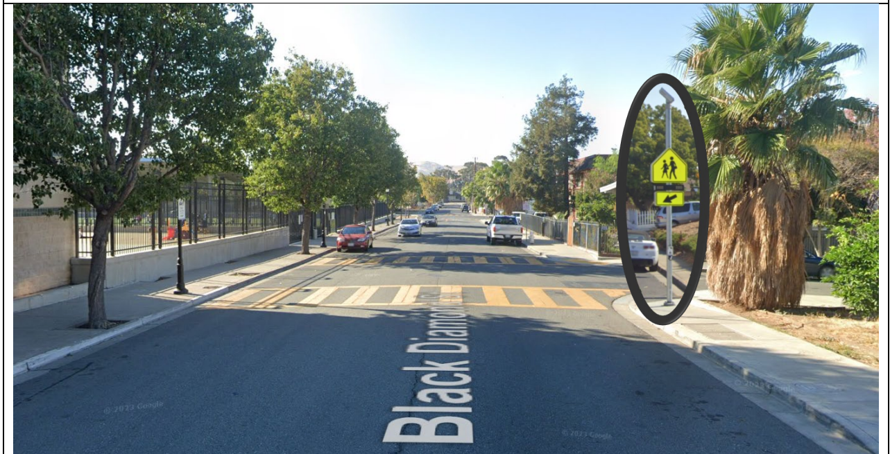
Example of Proposed RRFB to be Installed
