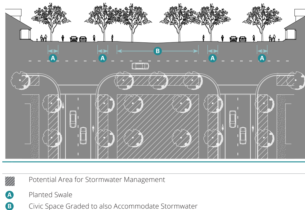
Figure 3.040.2 Stormwater Management Diagram
